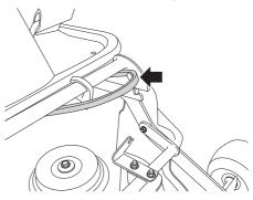
6 Loosen on the cutting height stay and place in the holder.
